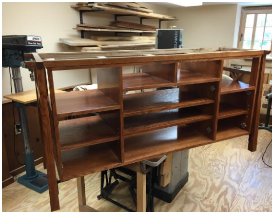
Figure 7. Table frame and cabinet assembly with shelves inserted prior to attaching cabinet doors.
