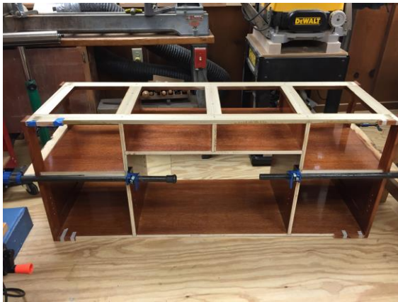
Figure 4. Cabinet takes shape with top formed with mortise and tenon joinery and horizontal and vertical boards positioned in dados for extra strength.
