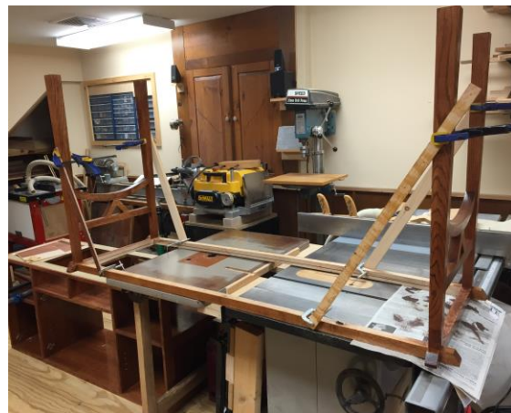
Figure 8. After final gluing, the upside-down table frame awaits an upside-down cabinet case for assembly.
