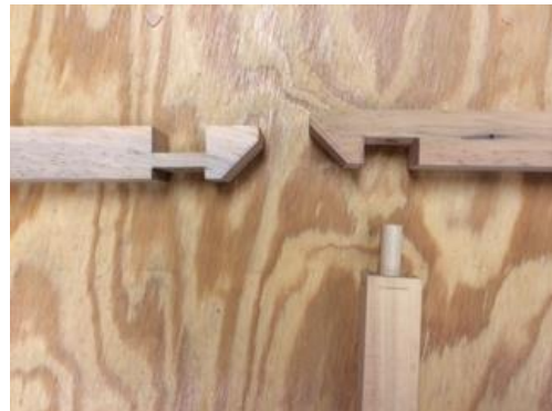
Figure 1. Components for interlocking table frame including leg (with dowel) was one of the clever woodworking features embedded in the design.
