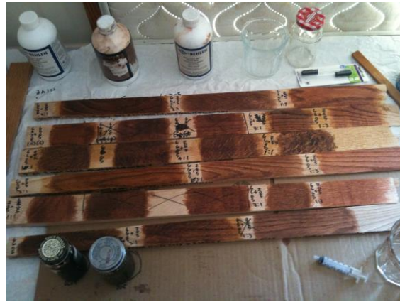
Figure 5. It took many attempts using a mixture of different Behlen NGR Solar-Lux stains on red oak samples to arrive at the desired color.
