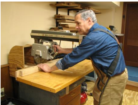
Figure 2. Jim demonstrating proper positioning for using radial arm saw.
